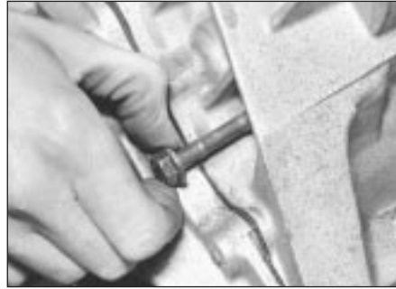
6.6a Undo securing bolts (recessed bolt shown) . . .
