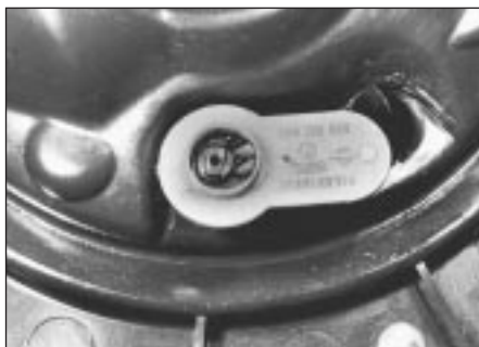
4.5 Upper view of air temperature sensor - 1.3 litre
