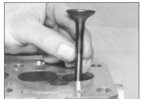
5.12 Removing a valve
