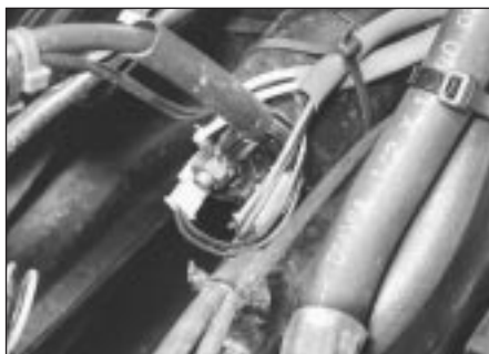
10.4 Starting motor solenoid wiring connections – 1.3 litre
