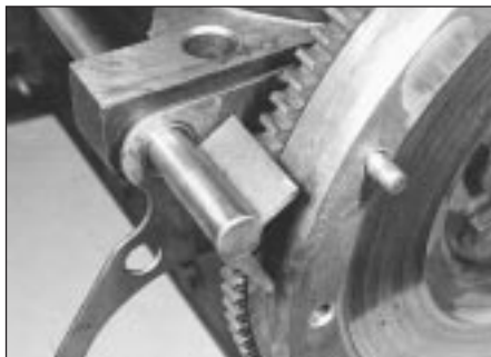
13.2 One method of holding the flywheel stationary
