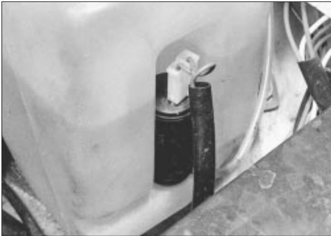
30.1 Windscreen washer pump and wire connector
