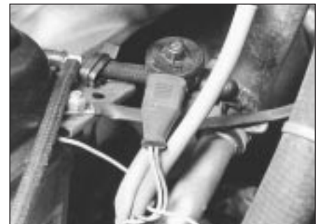
20.6 Fuel consumption gauge sender unit
