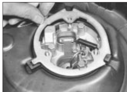
3.2 Removing air cleaner body retaining ring - 1.3 litre
