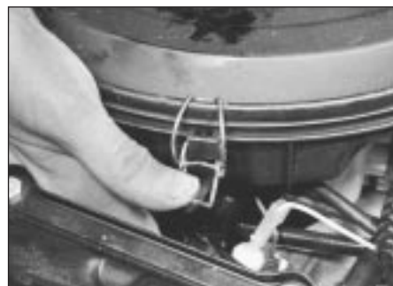
32.1 Unclip the air cleaner lid . . .
