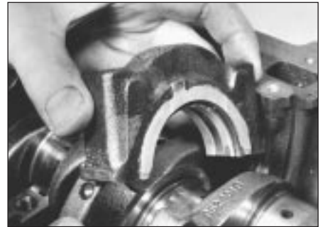
29.4 Fitting centre main bearing cap
