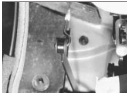
10.5 Accelerator cable-to-pedal attachment
