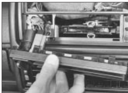
8.3b Unclip and withdraw trim panel
