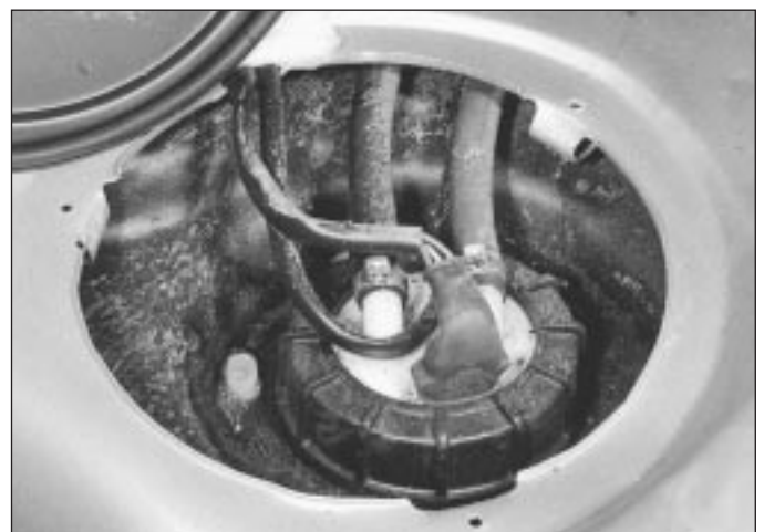
18.2 Fuel tank sender unit and connections
