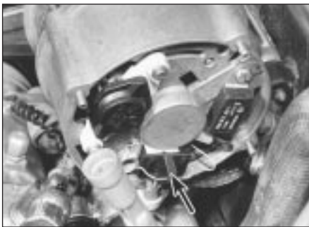
7.2 Lead multi-plug and retaining clip (arrowed) - Bosch alternator
