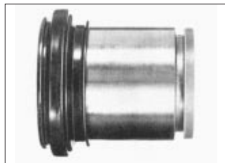
3.9 Dust seal location on caliper piston
