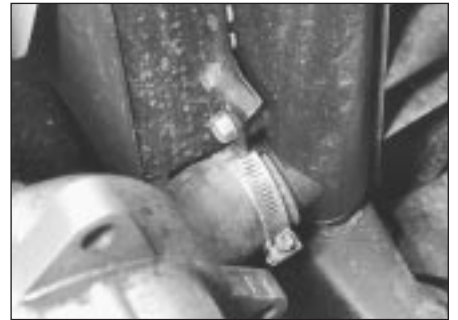
2.4b Radiator bottom hose connection - 1.8 litre
