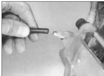
12.5 Connect bleed tube to bleed valve
