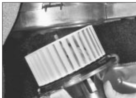
9.4 Blower unit withdrawal from housing
