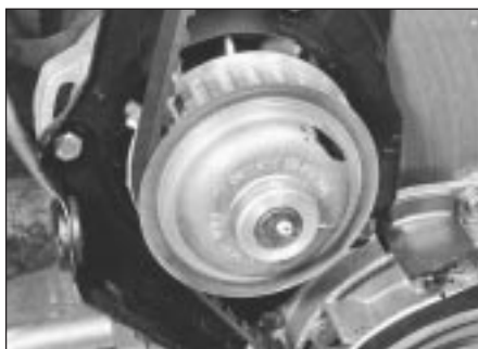
6.5 Disengage timing belt from coolant pump sprocket
