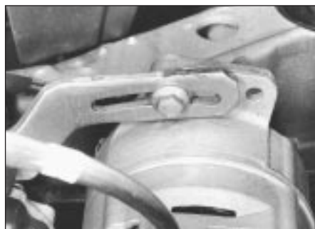
13.4a Alternator drivebelt tensioner link - 1.3 litre
