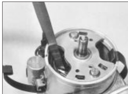
16.10a Checking contact breaker points gap
