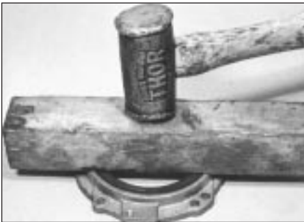
14.16 Installing new crankshaft rear oil seal
