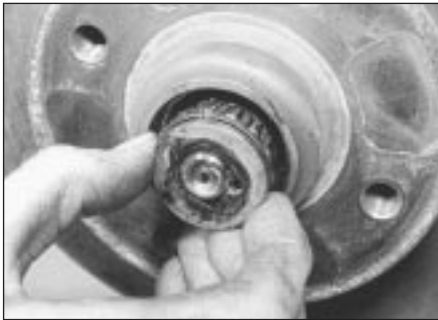
4.15 . . . followed by the outer washer and bearing
