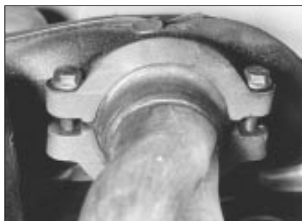
19.10 Exhaust downpipe-to-manifold flange connection - 1.3 litre
