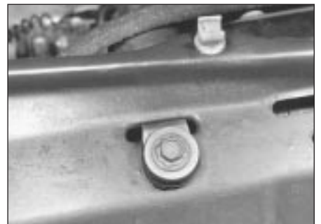
3.5 Radiator central retaining bolt and bracket
