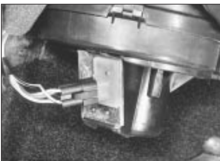
9.3 Blower unit and wiring connection
