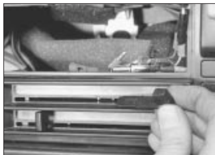
8.3a Pulling free heater/ventilation control knobs
