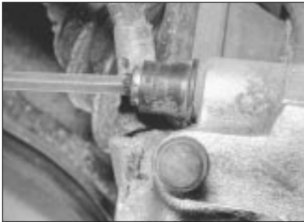
2.3a Caliper securing bolt removal
