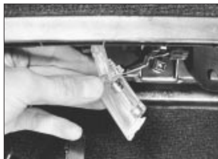
8.16 Luggage compartment lamp lens removal
