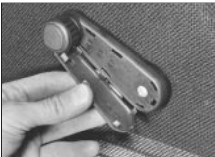
14.4a Remove window regulator handle cover . . .
