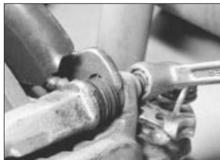
2.16 Rear caliper bolt removal
