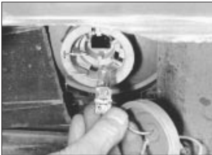
7.2 Bulb and holder removal from foglight
