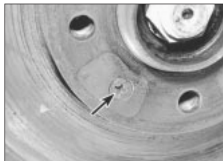
4.5 Front brake disc retaining screw (arrowed)
