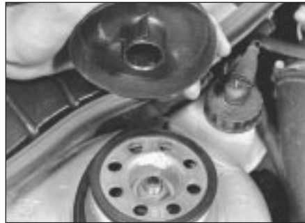
2.3 Removing front suspension strut top cap
