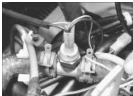
7.11 Temperature sender unit thermo-switch location - 1.05 and 1.3 litre
