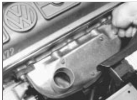
11.20 Fitting hot air shroud
