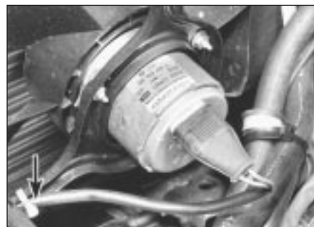
3.15 Secure fan lead with plastic clip (arrowed)
