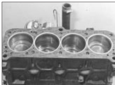
34.2 Cylinder head gasket located on block
