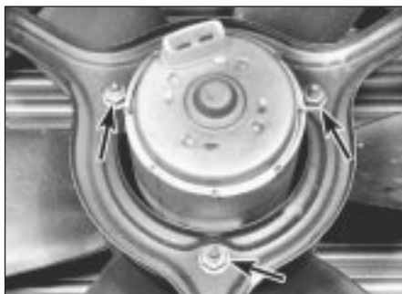
4.4 Cooling fan motor retaining nuts (arrowed)
