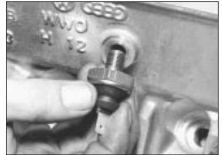
11.3 Refitting oil pressure switch
