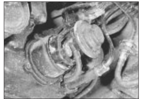
19.1b Fuel pump viewed from rear
