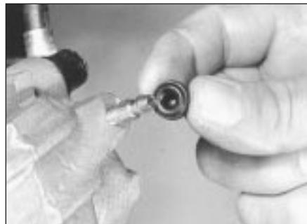
12.23 Fit bleed valve the protector cap
