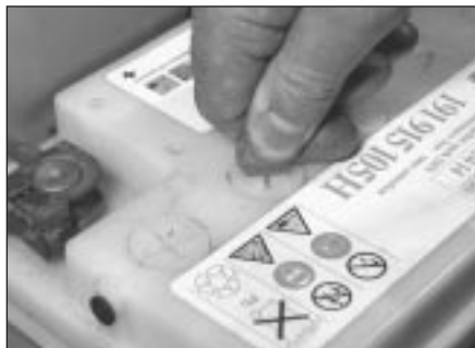
7.3a Remove battery filler caps . . .
