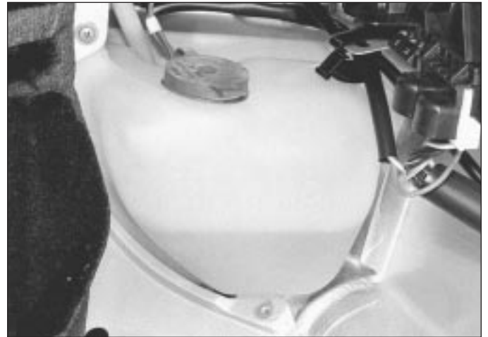
30.2 Rear window washer reservoir unit location
