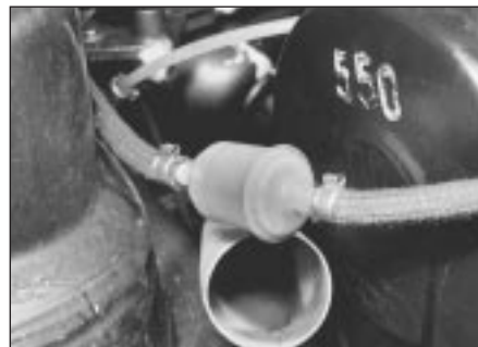
33.1 In-line fuel filter - 1.05 and 1.3 litre, carburettor
