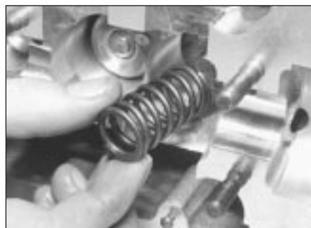
5.11b Removing an inner valve spring
