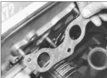
11.19 Fitting a new exhaust manifold gasket
