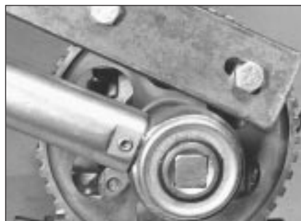
35.5 Method of tightening camshaft sprocket bolt
