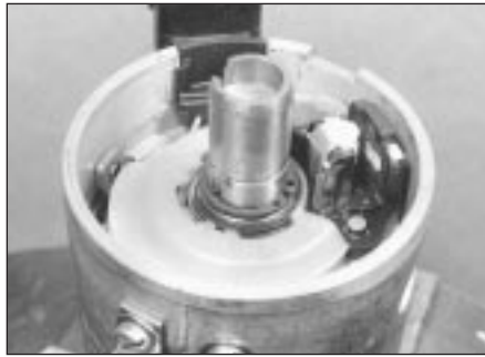
7.7 Hall sender unit, retaining ring and washers
