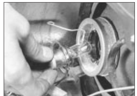
4.4 . . . and withdraw headlamp bulb
