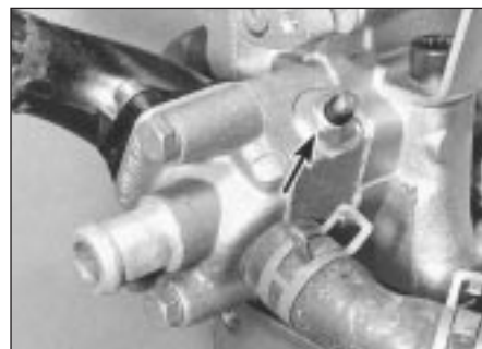
7.12 Temperature sensor (arrowed) - 1.05 and 1.3 litre
