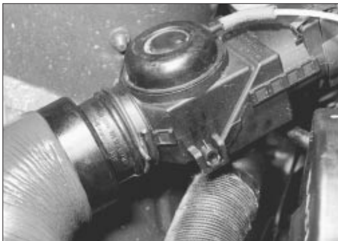
4.1 Air cleaner vacuum unit
