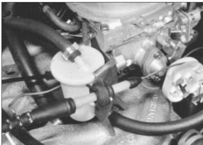
10.3 Accelerator cable to carburettor throttle control
