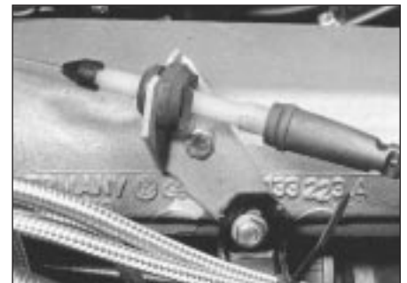
8.10 Accelerator cable adjuster and support bracket
