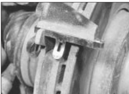
2.9 Pad retaining spring is located as shown
