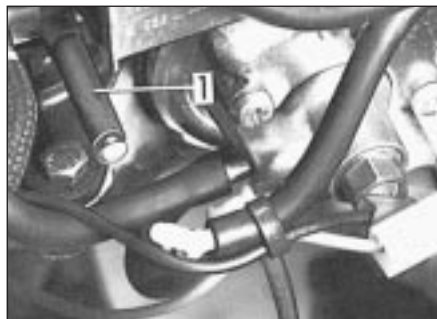
17.39a Disconnect and plug vacuum hose (1) to check/adjust engine fast idle speed adjustment
