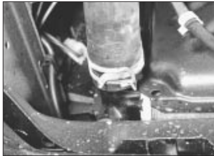
2.4a Radiator bottom hose connection - 1.3 litre
