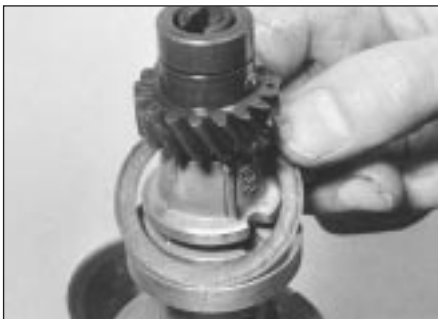
6.6b The gasket must be removed
