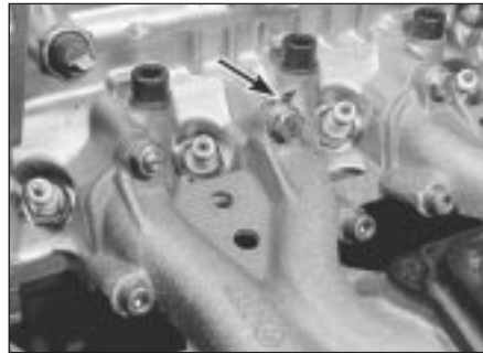
19.6 Inlet manifold-to-cylinder head securing nuts and bolts
