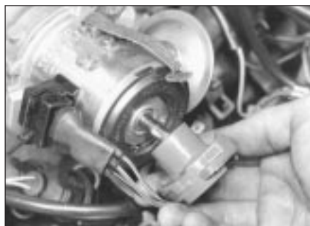
11.9 Fitting rotor arm
