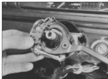
12.7a . . . and wiper control switch
