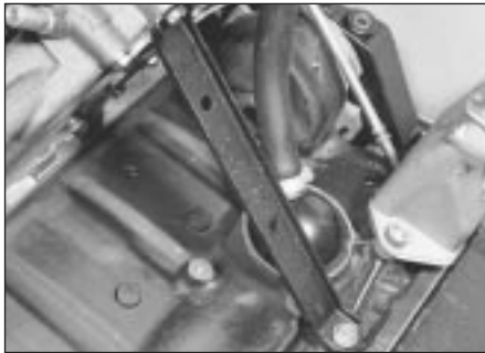
19.5 Inlet manifold support stay - 1.3 litre
