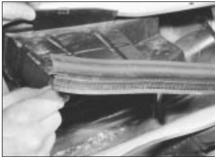
4.2a Carefully prise free plastic cover . . .
