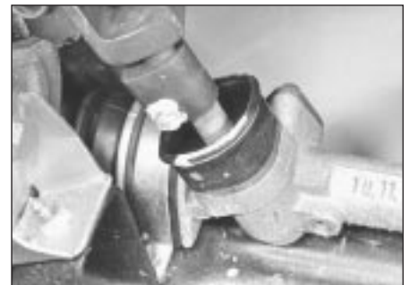
17.6 Steering gear pinion-to-lower column joint
