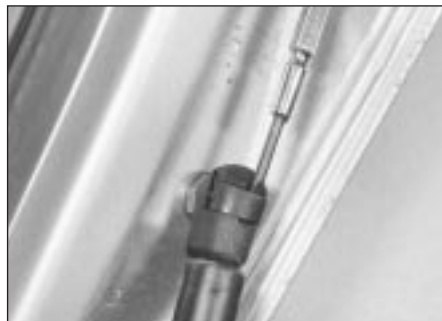
9.2a Releasing tailgate strut balljoint clip
