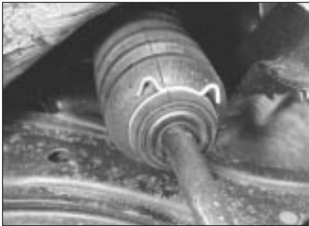
14.4 Steering tie-rod bellows and retaining clip
