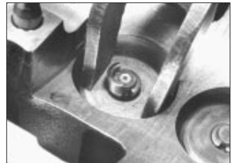
12.12c . . . and valve collets
