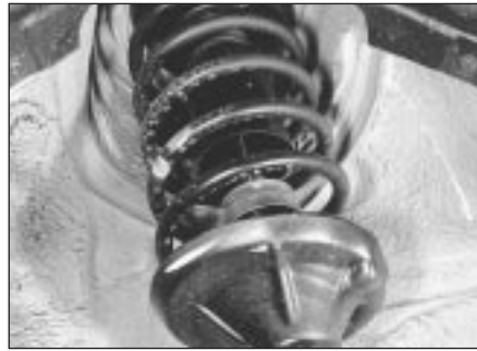
29.4 Check shock absorbers for leakage
