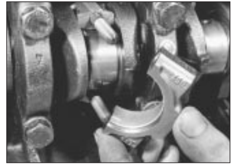
17.7 Withdrawing a big-end cap
