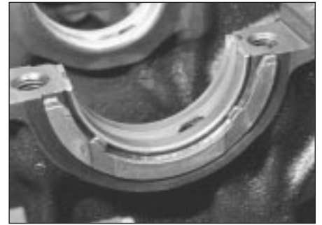
30.3c . . . together with thrustwashers
