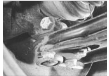
7.3 Track control arm balljoint and clamp bolt
